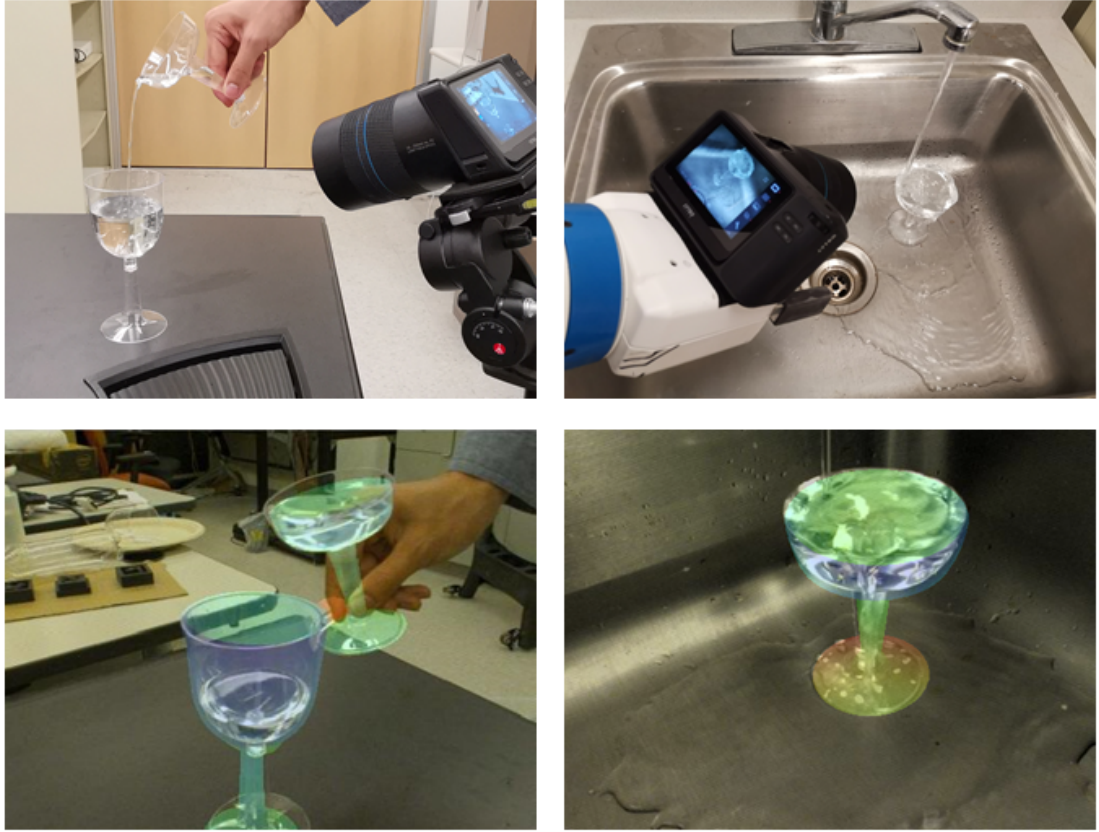
Figure 5.1: Demonstration of our LIT pipeline. (Top row) Lytro Illum camera is mounted on the tripod and robot arm to capture the transparent objects in challenging environments. (Bottom row) final estimated poses are overlapped to the center view of the observed light-field image.
