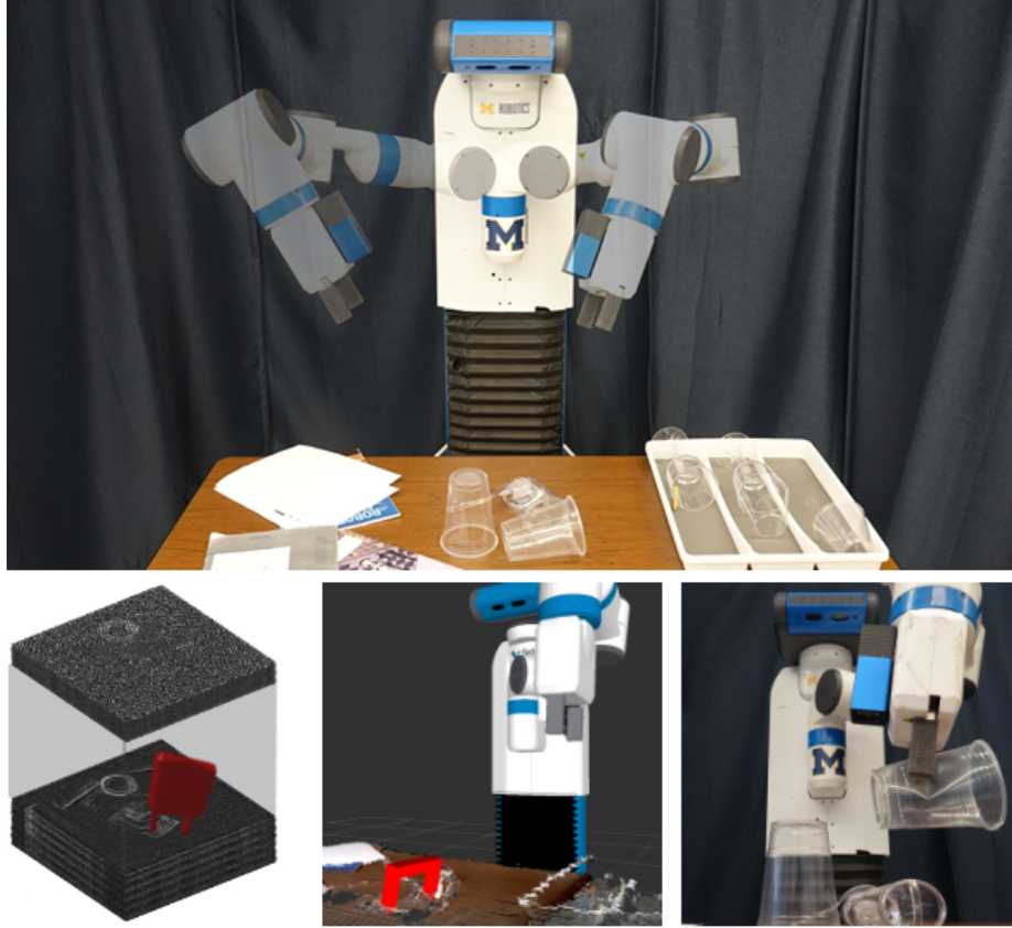
Figure 4.1: (Top) a robot using GlassLoc to pick up transparent objects from clutter and place on the tray. The robot is observing the scene using a light field camera. Grasp candidate is sampled in DLV (bottom left) and mapped to the world frame in the visualizer (bottom middle). The robot successfully picks up a transparent cup from the clutter (bottom right).
