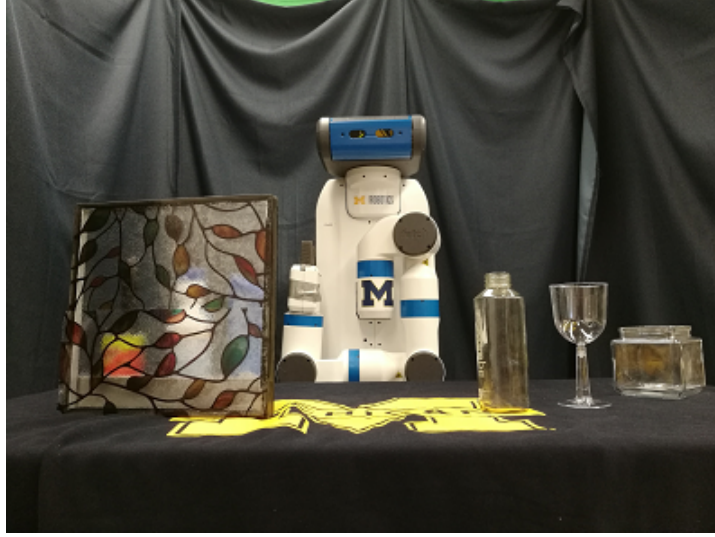
Figure 3.4: Test objects for evaluating PMCL 6D pose estimation include: (to the left) opaque objects behind a partially opaque translucent surface (a stained glass window film), and (to the right) transparent objects.
